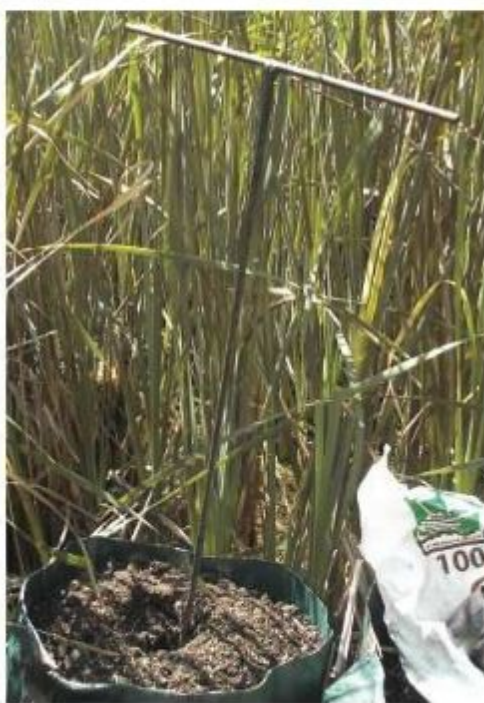
The custom mixing tool was welded together by a local blacksmith for $30 in materials and $20 in labor costs.
